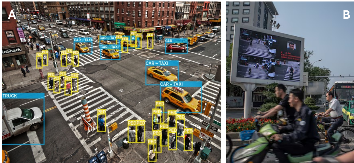
Fig. 1. AI-enhanced traffic surveillance systems: (a) AI analyzes traffic conditions and recognizes patterns of vehicles and pedestrians (Image courtesy: Travis Buckner); (b) A roadside screen displays jaywalkers, identified using AI, to deter violations (Image courtesy: Gilles Sabrié).
