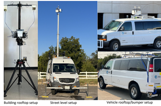
(b) Outdoor channel sounder mounted on vehicles
