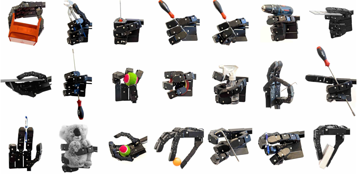
Fig. 4: The ISyHand performing a subset of grasps from the GRASP taxonomy [20].
