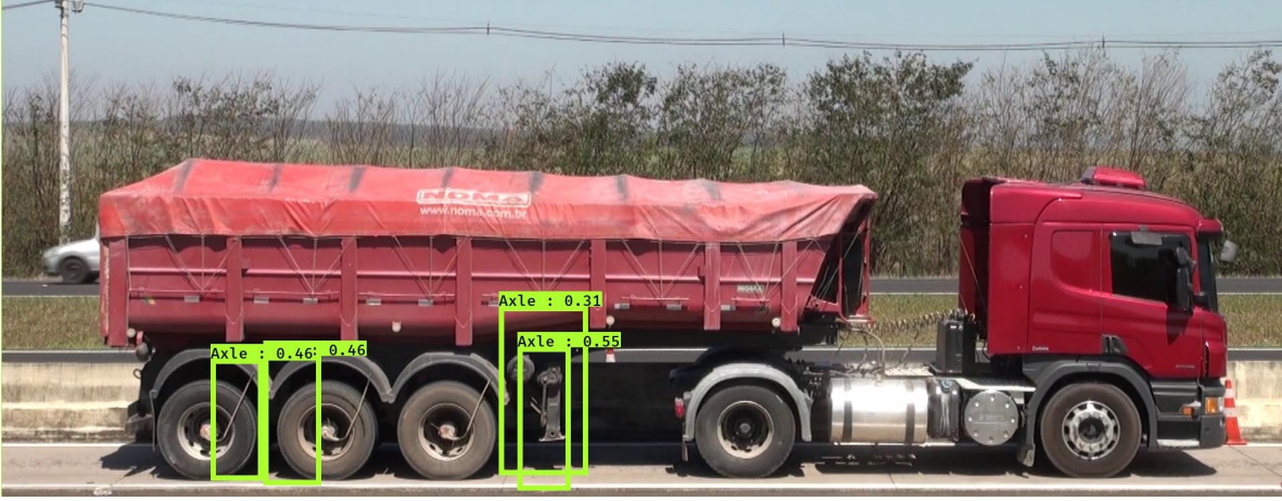
Figure 10: False negatives, when truck axles are not detected, and false positives, when objects that are not axles are detected and classified as axles.
