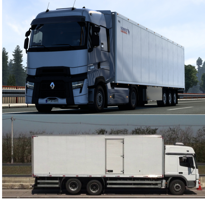
Figure 1: Example of synthetic and real-world data. The truck on the top is a rendered 3D model. The truck on the bottom is a real-life truck.
