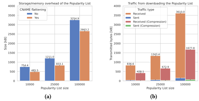
Figure 9: (a) Popularity List size in bytes as a function of N_{popular} , with and without CNAME flattening. (b) Total sent and received bytes to download the Popularity List (without CNAME flattening) over TLS, with and without compression.
