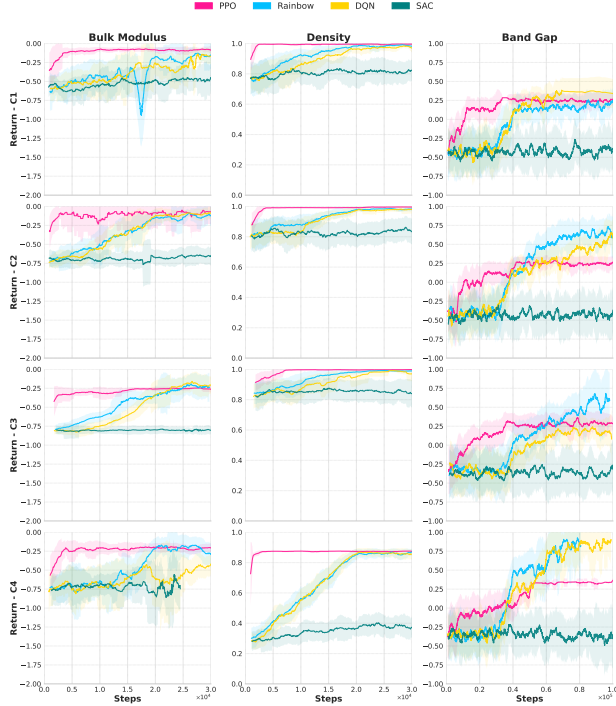
Figure 3: Learning curves for 4 of the 7 crystal structures in the simplest CrystalGym benchmark ( single structure, in-d. targets, small action space). Task difficulty varies with both property type and crystal structure.
