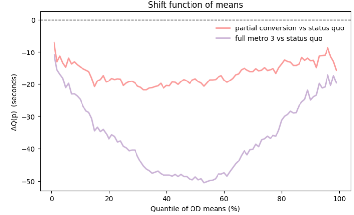
(b) Shift function of OD time distributions. For the entire distribution of OD times under each scenario, we compute the quantile function Q(p) of aggregated travel times and then plot \Delta Q(p) = Q_{\text{scenario}}(p) - Q_{\text{baseline}}(p) over p \in [1, 99] . Negative values denote time savings.
